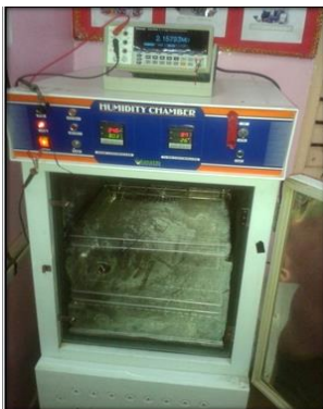
Figure 3: Experimental arrangement for humidity dependent resistance measurement.
