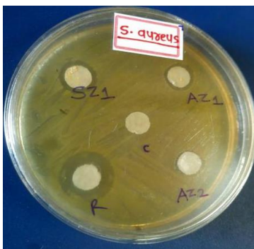
Fig.6. Antibacterial activity against gram positive S.aureus bacteria for ZnO nanoparticles.
